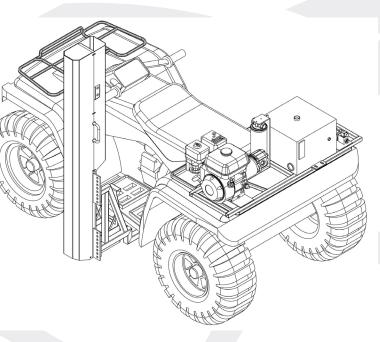
The operator will need to connect the hydraulic hoses from the power unit to the mast.
