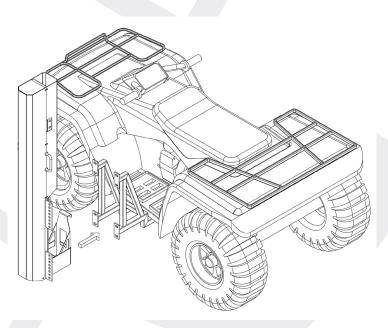
• The mast has multiple holes in the flange for the operator to adjust to the desired height. The recommended height from the ground surface to the bottom of the mast is 6". If the mast is mounted higher or lower than 6", a full 12" sample will not be collected. Eight bolting holes are provided on the mast mounting flanges, but only four 1/2" diameter bolts are needed to secure the mast to the mounting frame. Two bolts in the top flange and two bolts in the bottom flange.
