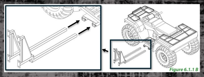
Secure the ATV & UTV Mast Mount using eight 3/8 in. diameter bolts. You may use the pre-welded nuts or drill new holes as needed. See Figure 6.1.1 C.
