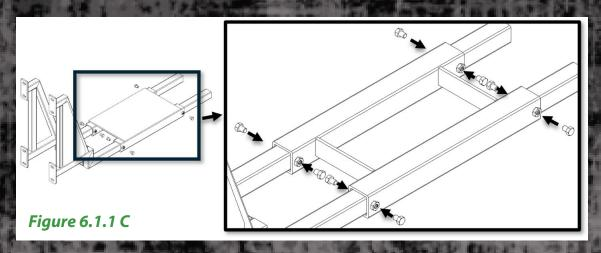
Attach the *Mast* to the ATV & UTV Mast Mount using the flanged bolt holes. See Figure 6.1.1 D.
